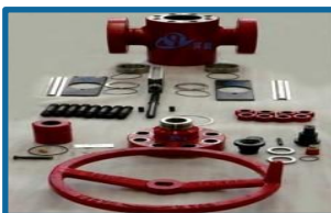
VALVES REPAIR & RE-CERTIFICATION
